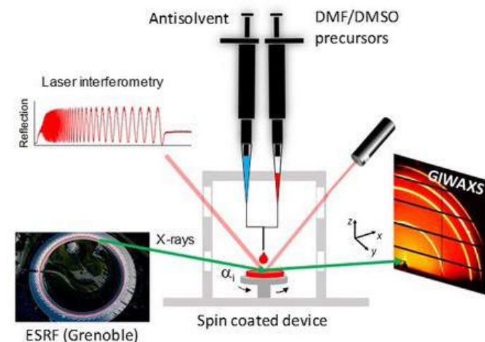
Scheme of the experimental setup used to investigate the structural formation of perovskites thin films during spin coating.
